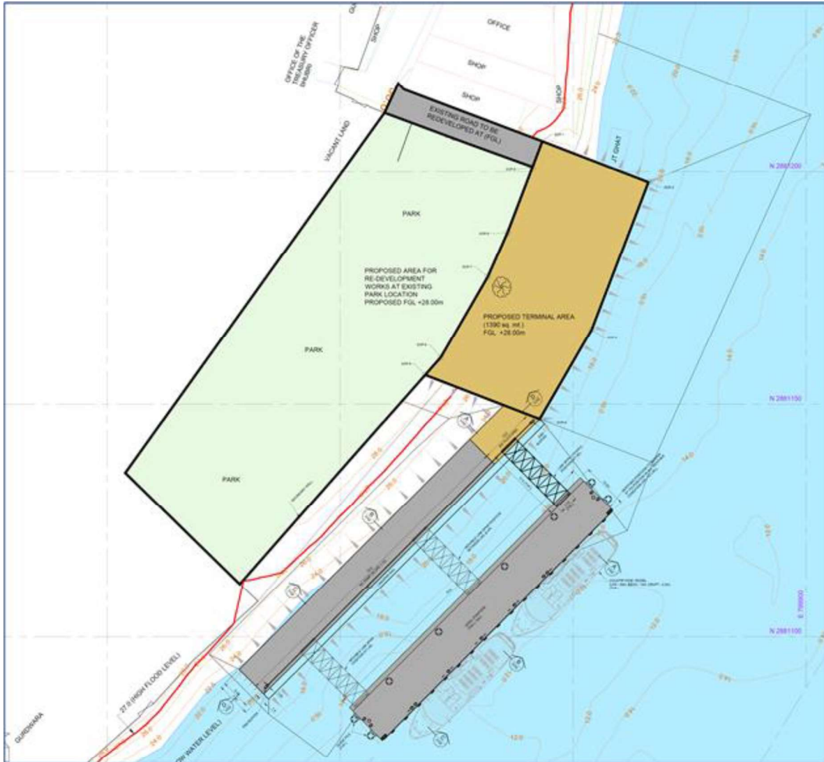
Figure 8-3 Concept solution 1b - Fixed multiple floating pontoons with the movable linkspan
