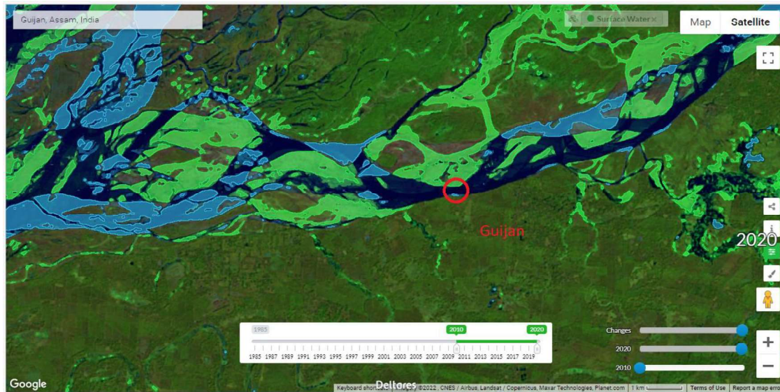
Figure 4-8 Aqua monitor images showing erosion and accretion changes from 2010 to 2020 ( https://aqua-monitor.appspot.com/ ) at Guujan (Blue colour polygon indicates: land has become water and green colour polygon indicates water has become land)
