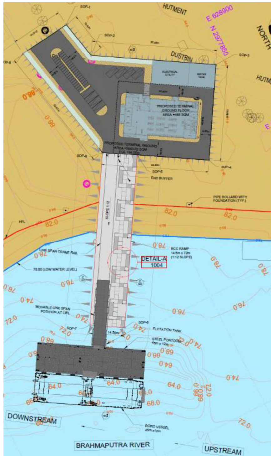
Figure 8-20 Plan view of approach bund connecting land side facilities with Linkspan setup
