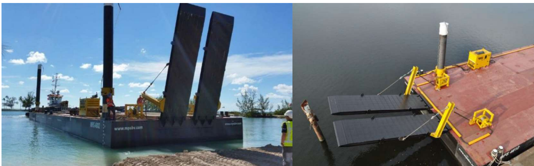
Figure 8-13 Concept Solution 5 - Spud pontoon
